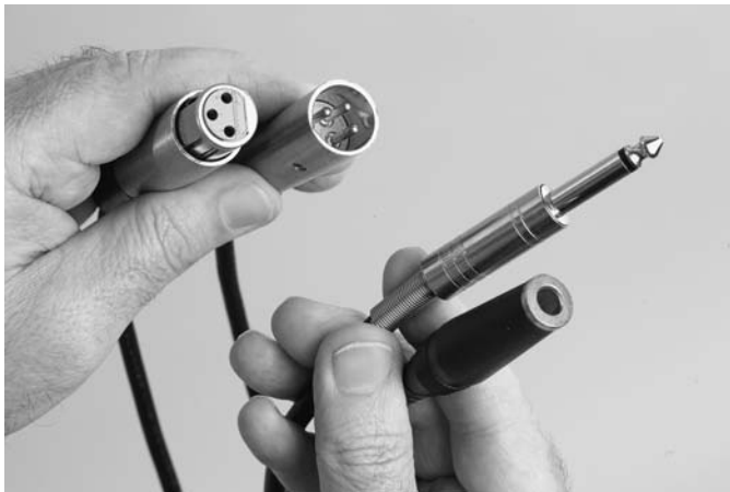
Figure 17-4: 3-pin XLR male and female connectors (left), and a 1/4-inch phone plug and jack (right).
