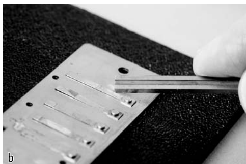
Figure 18-2: Embossing action along (a) the main part of the reed and (b) at the base of the reed.
