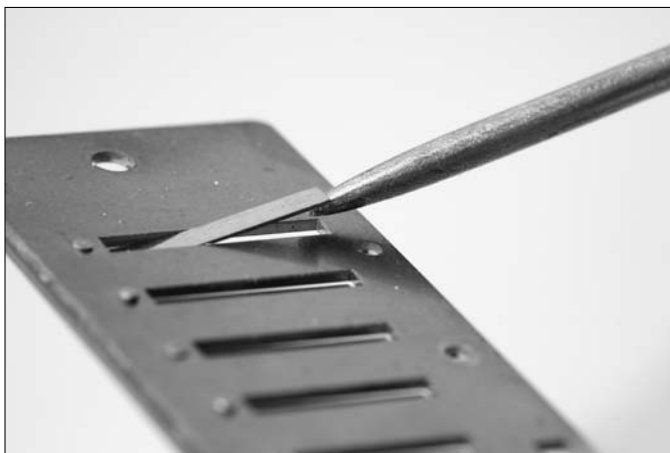
Figure 18-1: Flexing a reed through its slot to lower its action.
